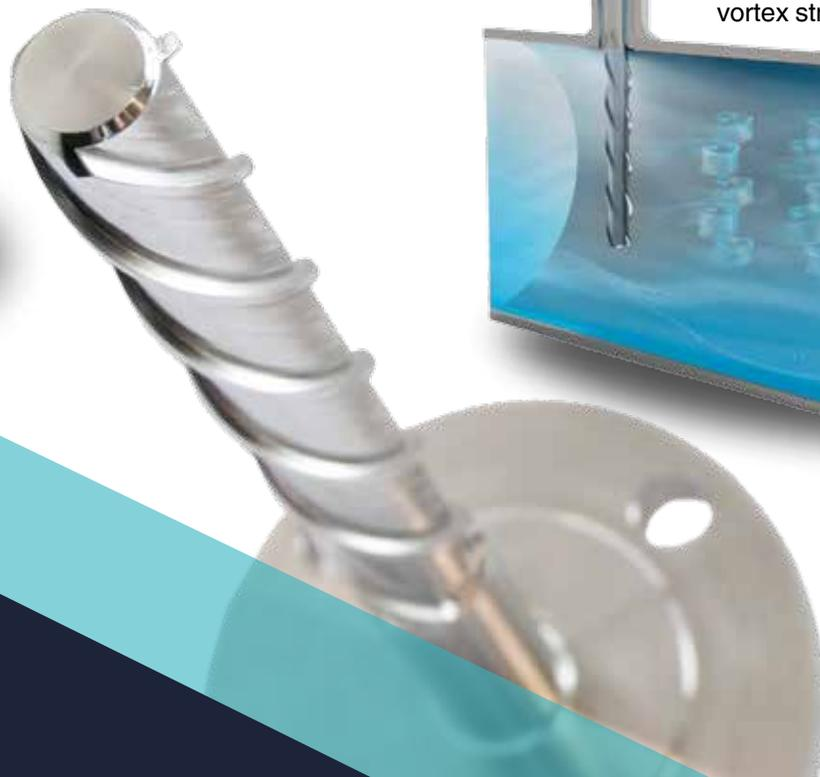
Helical coils break up the flow and thus impede the formation of a clearly defined Kármán vortex street
