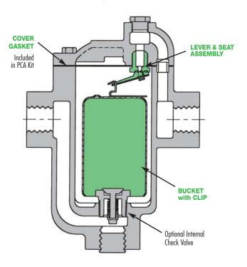
Replacement Parts & Kits for Inverted Bucket Steam Traps
