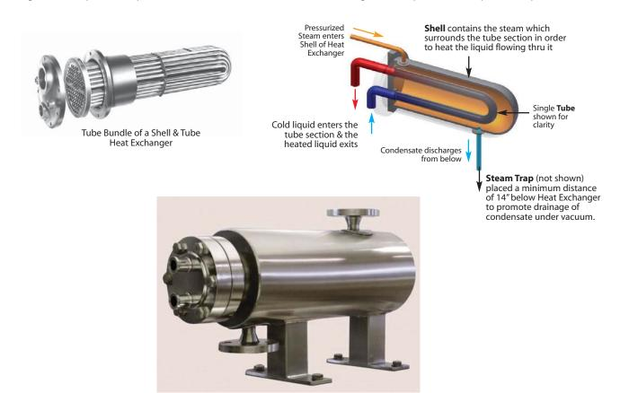
Shell & Tube Heat Exchanger
