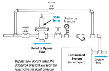
A Relief Valve allows water to recirculate through the pump even when the discharge valve on the pump is completely closed. As a rule, a minimum of 20% of the pump capacity must recirculate to prevent overheating of the pumped liquid.
