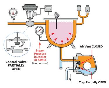
**Process Liquid is nearing Set Temperature**
