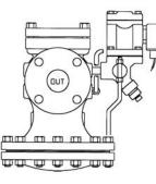
Shown with **PS** ON-OFF (solenoid Pilot) control pilot: The **PS** ON-OFF (solenoid) Pilot allows for the HD valve to be opened and closed using an electrical switch to activate a small solenoid valve. The **PS** Pilot can be used for system automation or as a safety shut down device. The ON-OFF pilot is most often used in conjunction with a Pressure or Temperature control pilot.
