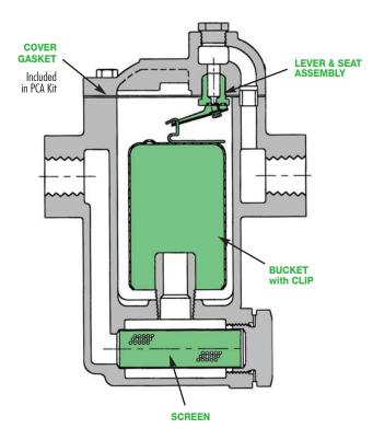
Inverted Bucket Trap 1032 shown with Check Valve
