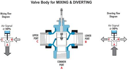
CAUTION: 3-Way Valves are not designed for use in steam applications. To properly control the mixing of two flows, inlet pressures at ports **B** and **C** should be as equal as possible.
