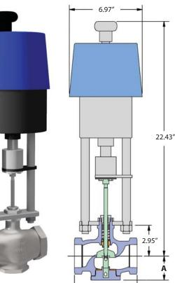
HB Series Control Valve (with Electric Actuator)
