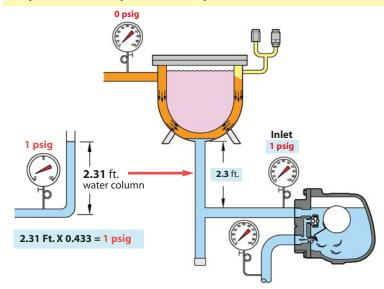
When set temperature of the process fluid is reached, the steam pressure inside the jacketed kettle may reduce to 0 PSIG or even go into Vacuum. To promote condensate drainage, the steam trap is placed a certain distance below the process equipment.
