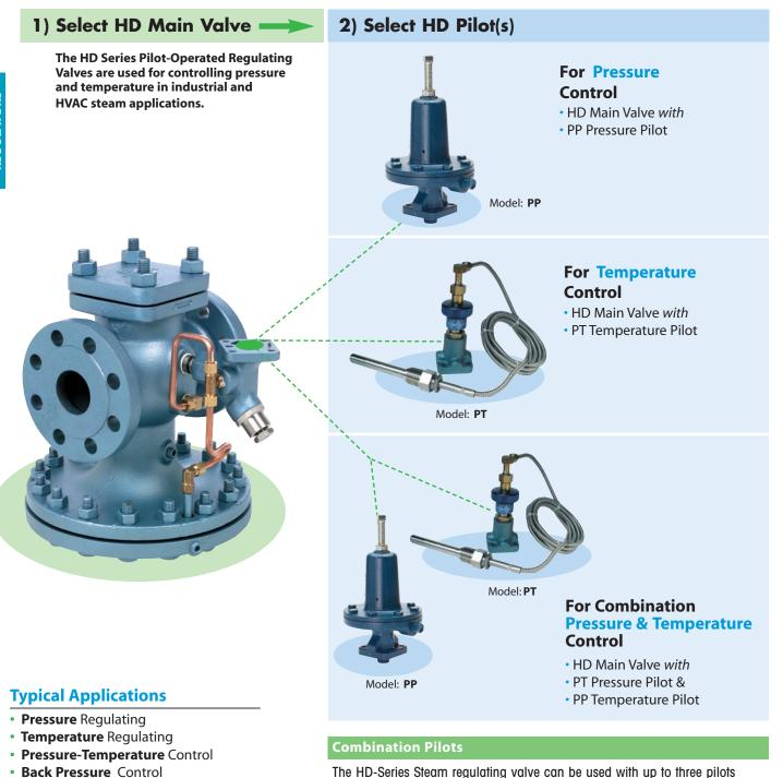
simultaneously to control the operation of the valve. An example is when steam is used to heat water in a Heat Exchanger. The Temperature Pilot will maintain precise control of outlet water temperature by controlling the amount of steam flow through the valve while a Pressure Pilot limits the maximum outlet steam pressure of the regulator to the Heat exchanger. A third pilot
