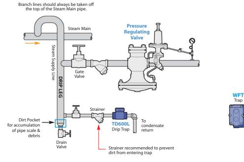
STEAM MAIN Isolation Valve Strainer To condensate return line Drain Valve
