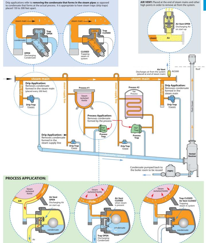
Process Applications refer to removing condensate and air from the actual process where steam is being used. This process could be a heat exchanger making hot water, or a radiator heating a room, or anything else that requires the use of steam. Traps used for process applications require larger condensate handling capability than steam traps used for drip applications and also need to be able to discharge large amounts of air.
