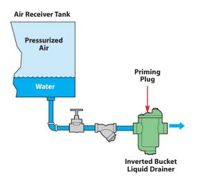
In an application where an Inverted Bucket Liquid Drainer is used, a balancing line may not be required. This style of drainer has a small internal bleed hole on the bucket float which allows a small amount of air to be vented. For the Inverted Bucket Liquid Drain Trap to operate, it must be primed with liquid prior to operation.
