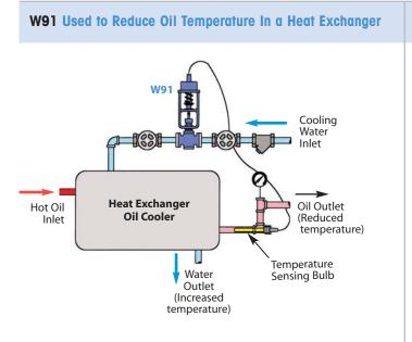
W91 Cooling valve controlling the flow of water through a heat exchanger to maintain the temperature of oil that is gaining heat by some process. The valve automatically shuts off when not required, greatly reducing cooling water usage. The source of the cooling water may be a well or city water supply and it can be circulated or dumped to drain. A 3-way valve may be used on cold water chiller systems so flow can be diverted from going through the heat exchanger when not required.
