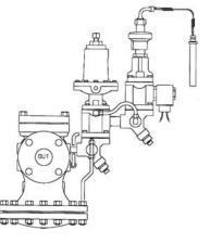
The **PT** Temperature Pilot will maintain the proper flow of steam through the main valve to keep the process it's controlling at the proper temperature as long as the **PS** ON-OFF (solenoid) Pilot is in the ON position. The **PP** Pressure Pilot will LIMIT the downstream pressure to a maximum value.
