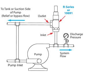
A Relief Valve allows water to recirculate through the pump even when the discharge valve on the pump is completely closed. As a rule, a minimum of 20% of the pump capacity must recirculate to prevent overheating of the pumped liquid.
