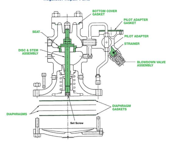
Pilots – HD Regulator Replacement Parts & Kits for Pilots used with HD Regulator
