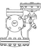
Shown with Air-loaded pressure control pilot. Air-loaded pressure pilots are used to reduce and control pressure in steam systems. They are used as an alternative to the more common spring-loaded pilot. The **PA** Air-loaded pressure pilot allows for remote adjustment of the valve using a small air regulator to alter the air pressure to the top of the pilot.
