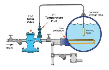
An overheat protection bellows is incorporated into sensing bulb.
