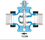
**Normally Open Valves** are used for **HEATING**, so the valve stem closes (**in-to-close**) as the control signal (temperature) increases.
