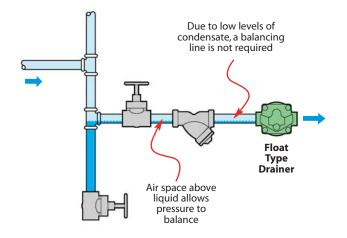
Typically, most air line applications have a low level of condensate to discharge, and the piping does not become flooded with condensate. In this type of application a Float Type Liquid Drainer can be used without the need of a balancing line. Due to the low level of liquid being drained, an air space exists above the liquid in the pipe which balances the pressure allowing liquid to flow freely.
