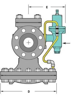
Standard pilot mounting is on the right side of the regulator when looking into the outlet port (as shown). Pilot mounting on HSP regulators are field-reversible.
