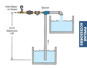
The maximum height that water or any liquid with a specific gravity of 1 can be lifted is 25 feet. Increases in the temperature of the liquid being lifted will cause this maximum height to decrease. Pumping liquids in excess of 130°F is not recommended. Please consult factory with any specific application.
