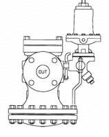
Shown with **PP** Pressure control Pilot. Spring-loaded pressure pilots are the most typical method of controlling downstream pressure in Steam Systems. Adjustment screw on top of pilot controls downstream steam pressure.
