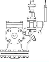
The **PT** Temperature Pilot will maintain the proper flow of steam through the main valve to keep the process it's controlling at the proper temperature as long as the **PS** ON-OFF (solenoid) Pilot is in the ON position. Available in either Normally-ON or Normally-OFF configuration; an electrical signal turns valve OFF or ON.
