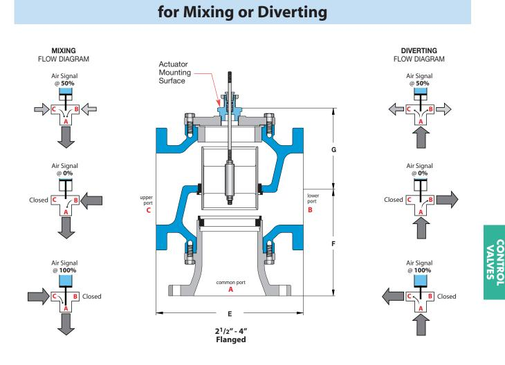
CAUTION: 3-Way Valves are not designed for use in steam applications.
