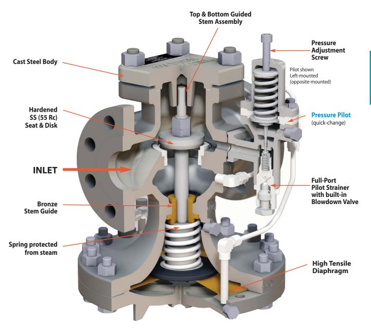
Pressure Regulator shown with Left-mounted Pilot (right-mounted is standard) Model includes HSP Main Valve with Pressure Pilot
