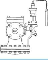
Shown with Temperature control Pilot: The **PT** Temperature Pilot will control the flow of steam flowing through the HD valve based on the temperature of the sensing bulb. The liquid-filled sensing Bulb is available in standard 8 ft and 15 ft capillary lengths. Other lengths available.
