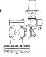
The **PP** Pressure Pilot will maintain the desired downstream set pressure as long as the **PS** ON-OFF (solenoid) Pilot is in the ON position. Available in either Normally-ON or Normally-OFF configuration; an electrical signal turns valve OFF or ON.
