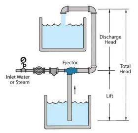
It is always desirable to keep the Ejector as close to the actual liquid being pumped as possible. The maximum height the liquid can be pumped depends upon the pressure of the "motive" liquid or steam available. Please refer to the capacity graphs for maximum flow rates and maximum achievable heads.
