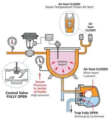
**Temperature of Steam causes Air Vents to Close**
