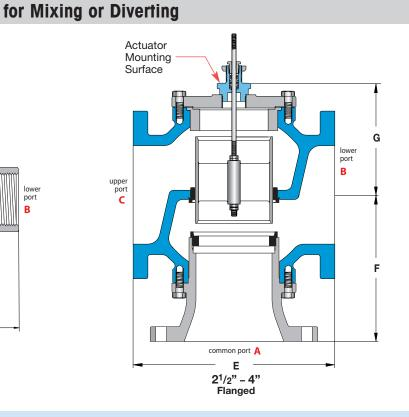
**CAUTION:** Watson McDaniel 3-Way Valves are not designed for use in steam applications. To properly control the mixing of two flows, inlet pressures at ports B and C should be as equal as possible.
