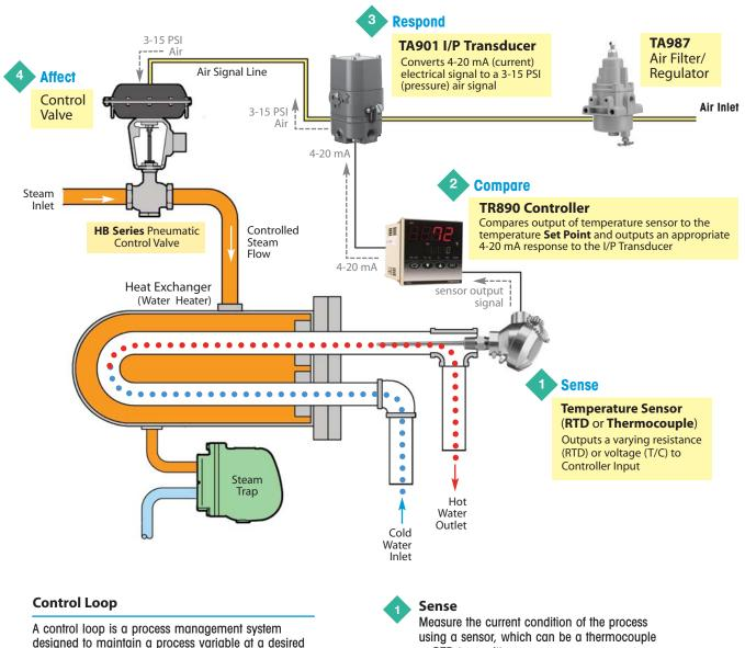
A control loop is a process management system designed to maintain a process variable at a desired set point. Each step in the loop works in conjunction with the others to manage the system. Once the set point has been established, the control loop operates using a four-step process.
