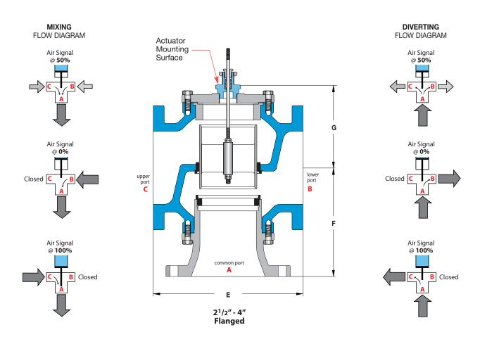
CAUTION: 3-Way Valves are not designed for use in steam applications.
