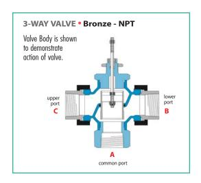
for MIXING & DIVERTING • Water & Other Liquids
